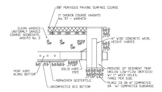
12. A weir plate or weir within an inlet or overflow control structure may be used to maximize the water level in the stone bed while providing sufficient cover for overflow pipes.
