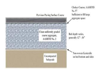
Pervious pavement consists of a permeable surface course underlain by a uniformly-graded stone bed which provides temporary storage for peak rate control and promotes infiltration. The surface course may consist of porous asphalt, porous concrete, or various porous structural pavers laid on uncompacted soil.
