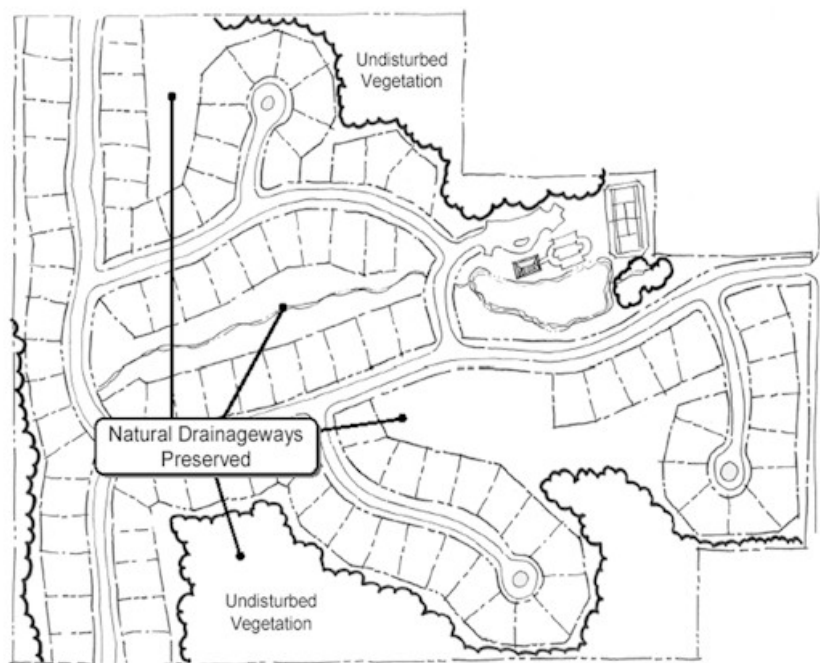
Figure 5.3-1 Protect natural drainage features
