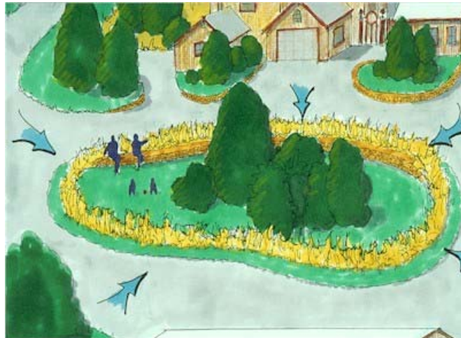
Figure 5.3-6 Natural surface depressions can temporarily store stormwater.
