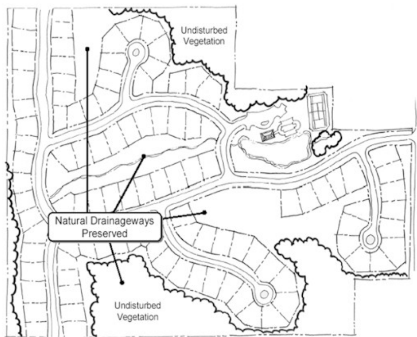
Figure 5.3-1 Protect natural drainage features
