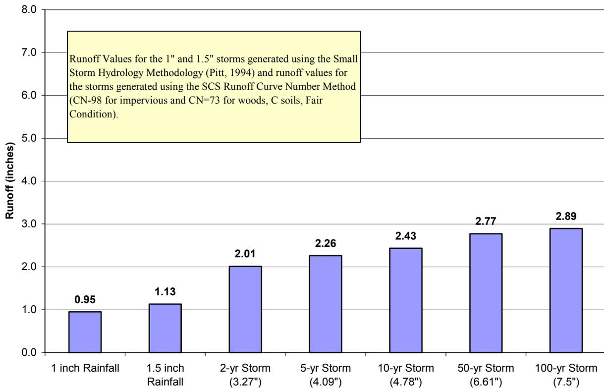
**Figure 3-2. Runoff Volume Increase from Impervious Surfaces - C Soils**
